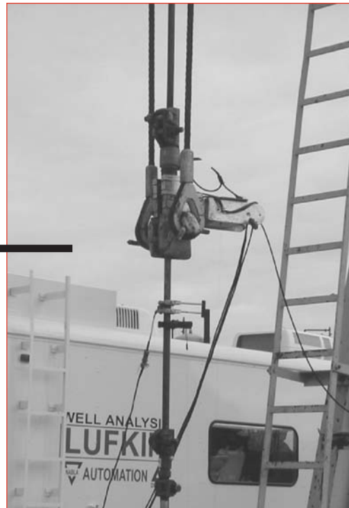
Figure 3. Experimental arrangement showing, 1) POC polished rod load cell, 2) horseshoe load cell for the SAM Quick Dynamometer, 3) horseshoe load cell and string position transducer basket for comparison with the PAIL Dynamometer, 4) clamp-on load transducer for the SAM Quick Dynamometer, and 5) string transducer clamp for the SAM Quick Dynamometer.
